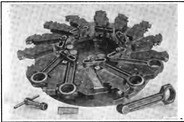
Fig. 15. Continuous Milling Fixture for Liberty Motor Connecting-rods
